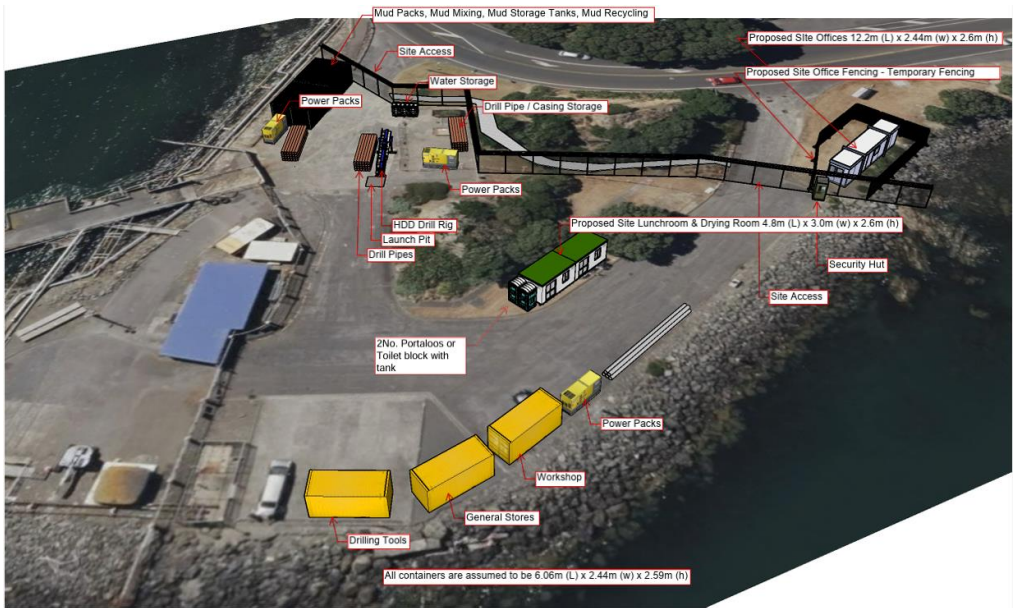
Figure 3: Temporary Construction Buildings for HDD Methodology
