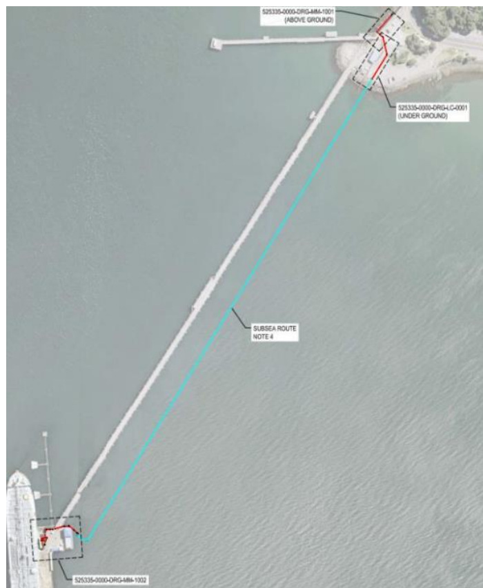
Figure 1: Proposed works sections from application. Turquoise = submarine pipeline, red = riser, spool and onshore pipe
